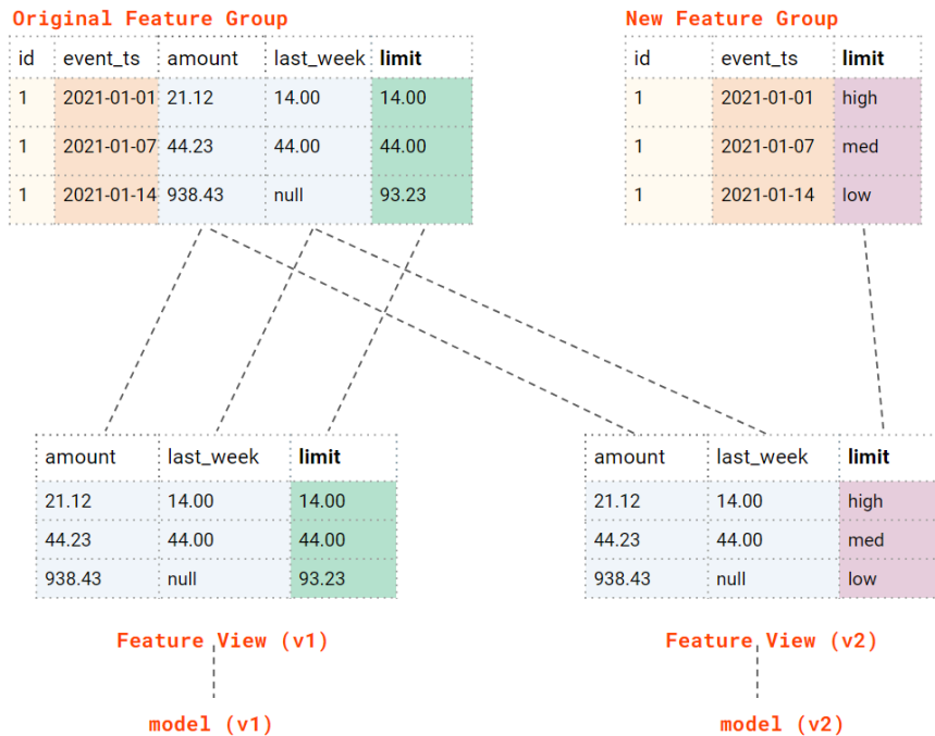
Figure 5-8. “New Feature Group” stores a categorical version of the “limit” feature - the original is a numerical feature. Feature View (v2) replaces the old limit feature with the new one, but keeps the other features unchanged from v1. Model (v1) continues to use the old “limit” feature, while model (v2) uses the new “limit” feature.
