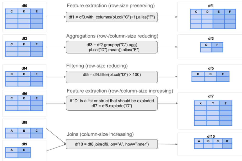
Figure 6-3. Data transformations produce output DataFrames that often do not match the shape of the input DataFrame(s). Some transformations add rows and/or columns, some keep the same number of rows, and some reduce the number of rows and/or columns.
